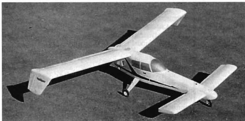
The Canada Goose canard features stressed-skin construction. Power is a .35ci engine.
