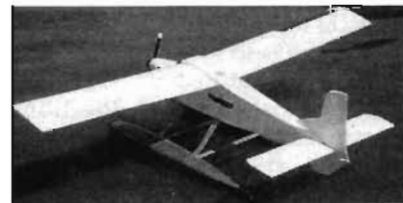
Powered by a .45 converted to diesel operation, Osprey was designed as a trainer with 3 degrees of dihedral, slotted flaps and a generous dorsal fin. CLA was at 25 percent of the VTMA, and tail-dragger landing gear was used. It was a stable, yet maneuverable model to fly. Banked 15 to 20 degrees and controls neutralized, it would return to upright level flight in about 90 degrees of a circle. Flaps down, it was stable, and on floats, it was pure fun.
