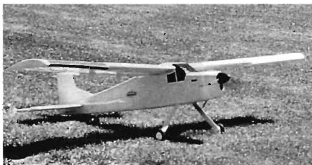
The Osprey, powered by a .45 diesel, about to start its takeoff run. The leading-edge droop shows clearly.
