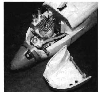
Photo D. This cowl detail shows that servicing the engine is easy.
