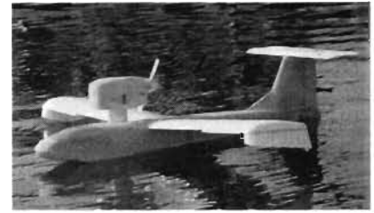
Seagull III. The original design had the engine nacelle farther back. The "balancing act" indicated that it was tail heavy. The nacelle was moved forward 2 inches; no ballast was needed when the model was completed.
