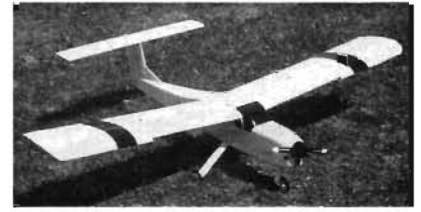
The Snowy Owl has an external glow-plug power plug in the jack. Plug removal is safely away from the dangerous rotating prop. It's .40ci powered.
