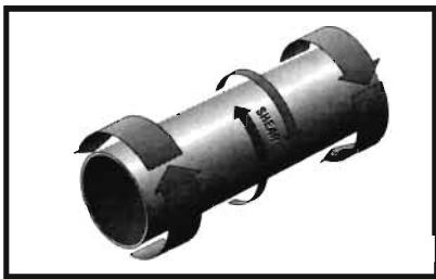
Figure 4. Tube under torsion.
