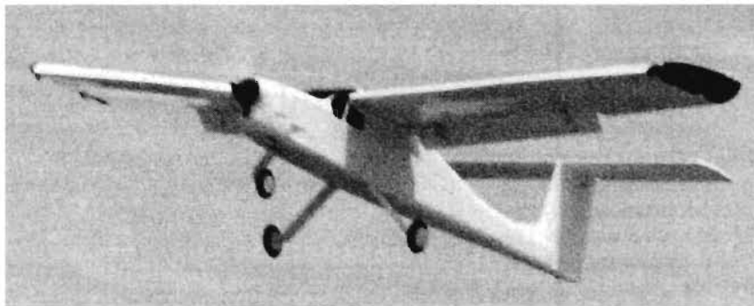
The Snowy Owl in slow-speed flight with flaps extended. The increasing leading-edge droop ahead of the ailerons is clearly visible.
