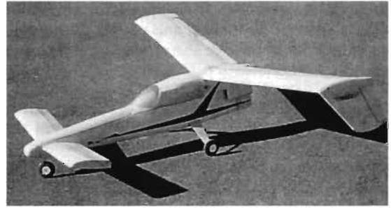
The Canada Goose Canard's tricycle landing gear. Propeller clearance on takeoffs and landings is critical for rear-engine canards.
