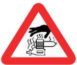
Model motors and their exhaust systems become very hot when running. Do not touch any part of the motor or exhaust, and keep well clear of hot exhaust gases and liquid combustion residues, as they can cause serious burns. Don't touch any part of the motor or its exhaust system until they have cooled down to ambient temperature.
