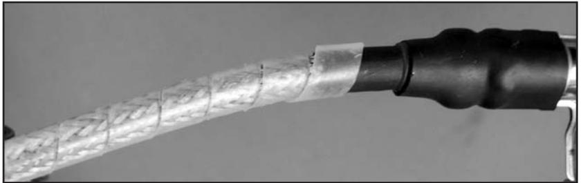
7. Install the remaining silicone wire cover over the ignition wire.
