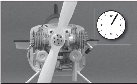
**4.** Place the propeller on the crankshaft at the one o'clock position.
