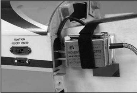
6. Install the ignition module and battery securely in the airplane forward area. It is recommended that a thin piece of foam rubber is placed between the module and the mounting surface and that Velcro® strap is used to hold the module in place.
