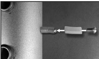
11. If not being used, plug the smoke fitting on the muffler with a segment of fuel tubing and an 8-32 screw (not included).
