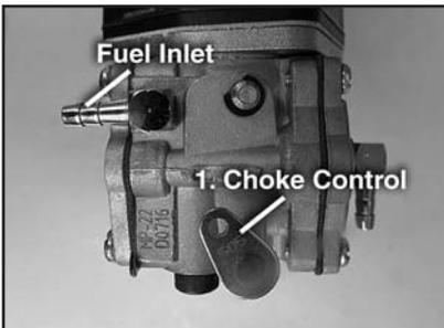
6. Install the choke servo (optional) at least 305mm [12"] away from the engine. Be sure to use a non-metallic linkage.
