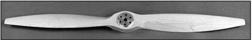
2. Once the location is established, use a drill press with a #5 (.2055" / 5.21mm) drill bit as a pilot hole. Once the pilot hole is established use a 13/32" (.406/10.31 mm) drill bit to finish the hole. In order to achieve a clean opening on both sides of the propeller, drill only half way through the propeller with the finishing drill bit. Then flip the propeller over and drill completely through the hole.
