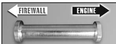
4. Install the 4 standoffs to the engine in the orientation shown using the (4) 5x20mm SHCS and 5mm washers. Be sure to use threadlocker.
