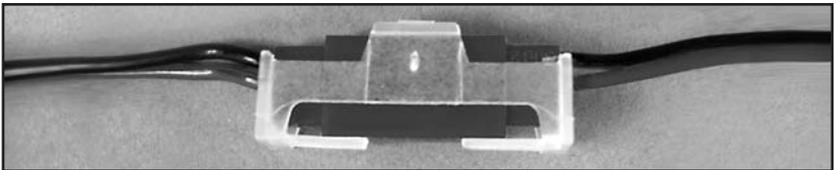
3. Connect the manual on/off switch lead to the red connector from the electronic ignition system using the lead from the kill switch or with the included three pin connector with pig tail. Use one of the included three pin securing clips to secure the connection.
