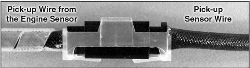
2. Install the silicone wire cover over the pick up lead coming from the engine (cut the excess silicone wire cover) and connect the lead to the pick-up lead from the Electronic Ignition Module. Secure the connection with the included three pin connector securing clip.
